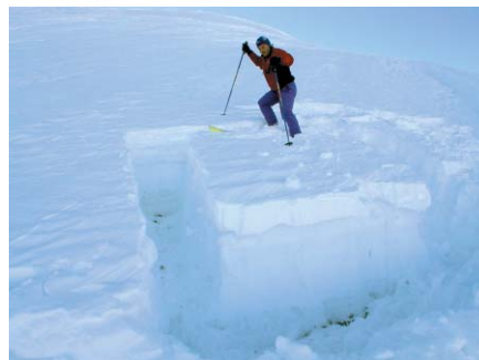
Figure 2.22 - Execution of slide block test - Rutschblock - to assess the resistance of the snowpack to cutting
