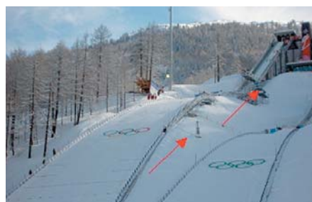
Figure 2.54 - Sonic anemometers installed along the ridge between the two ski jumps
