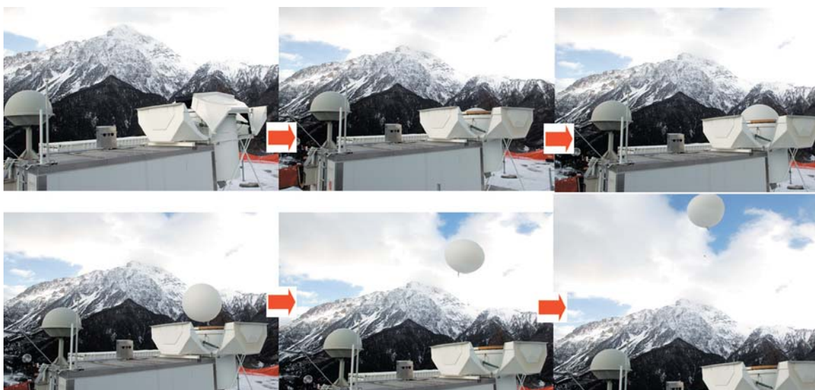
Figure 2.45 - Radiosonde launch system at Cesana Pariol
