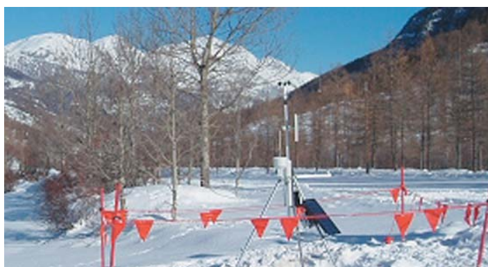
Figure 2.64 - Portable weather station at the lowest point of the course, which varied depending on the competition course, requiring the movement of the portable station as and when necessary
