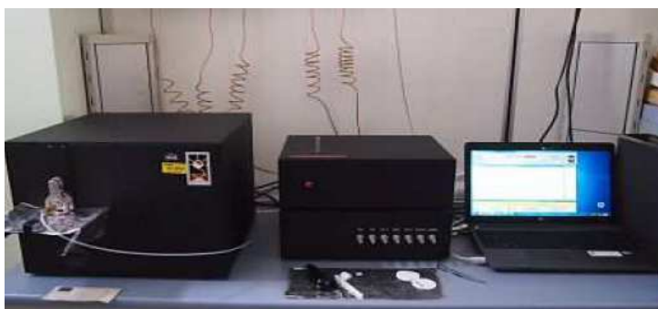
ANALIZZATORE TERMO-OTTICO TOT/TOR ( Thermal-Optical Transmittance/Reflectance ) OCEC Dual Optical Lab Instrument – Sunset Laboratory Inc. ARPA Piemonte – Lab. Grugliasco (TO)
