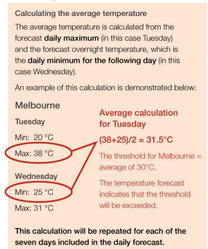
Figure 2: Example calculation of the daily average temperature
